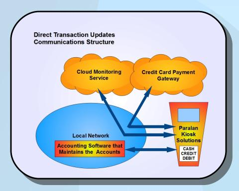
All Paralan Kiosk Solutions kiosks are remotely monitored, and designed for complete cloud control of the payment center. This is the new way that kiosks are being monitored, and updated. No longer does servicing the payment kiosk require going on-site to troubleshoot, or to reset the kiosk.
